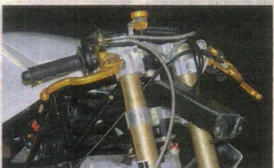
Fork-mounting system has two separate steering shaft bolts
