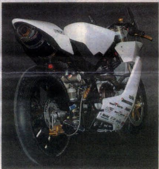
Wheels and tyres are from a 125cc machine, to save weight
